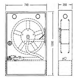
Standard assembly includes brass inductor, fibreglass foam tank and mild steel reel. Other materials of construction are available on request.
